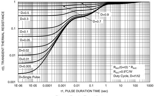
Figure 13. Transient Thermal Resistance
