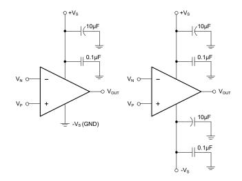
Figure 3. Amplifier Power Supply Bypassing
