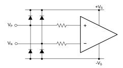
Figure 1. Input Equivalent Circuit
