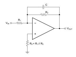
Figure 6. Active Low-Pass Filter
