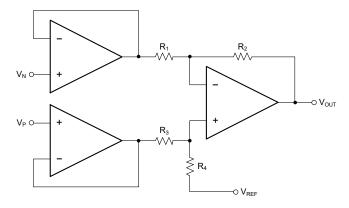
Figure 5. High Input Impedance Difference Amplifier
