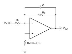
Figure 6. Active Low-Pass Filter
