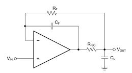
Figure 2. Circuit to Drive Heavy Capacitive Load
