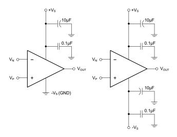
Figure 3. Amplifier Power Supply Bypassing
