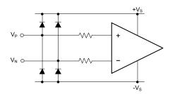
Figure 1. Input Equivalent Circuit
