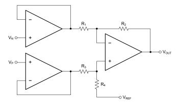
Figure 5. High Input Impedance Difference Amplifier
