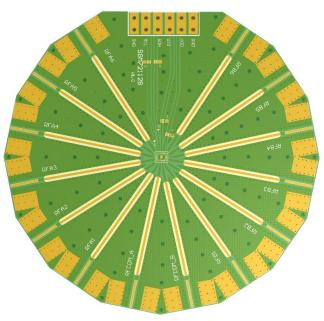
Figure 5. SGM72112B Evaluation Board Layout
