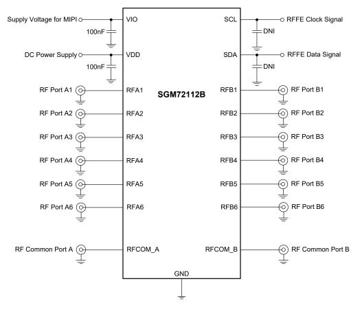
Figure 4. SGM72112B Typical Application Circuit
