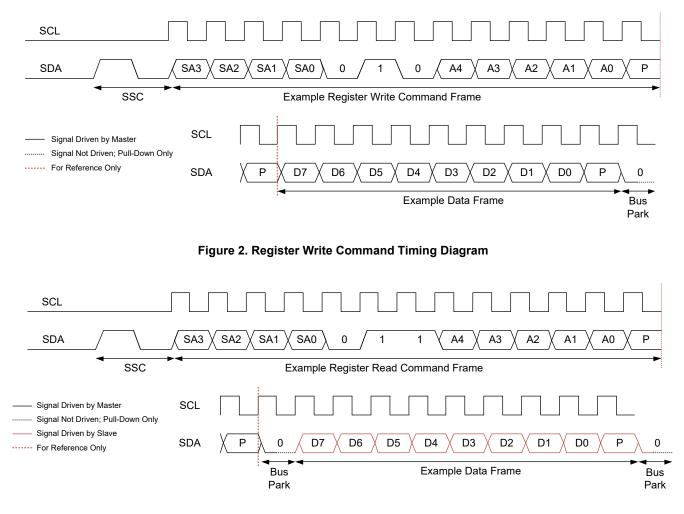
Figure 3. Register Read Command Timing Diagram
