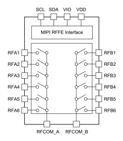
Figure 1. SGM72112B Block Diagram
