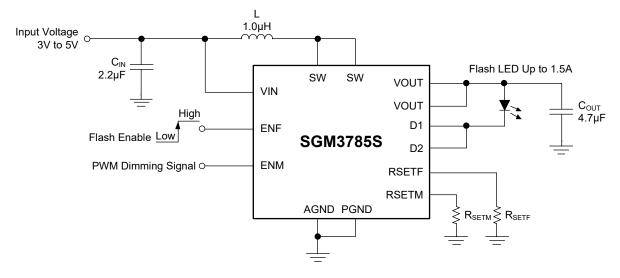
Figure 3. Typical Application of Flash Mode
