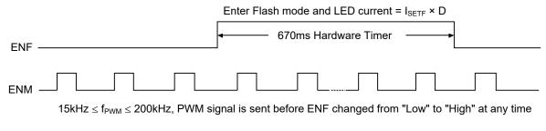
Figure 4. Timing Diagram of Flash Mode
