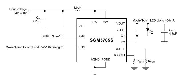
Figure 5. Typical Application of Movie/Torch Mode
