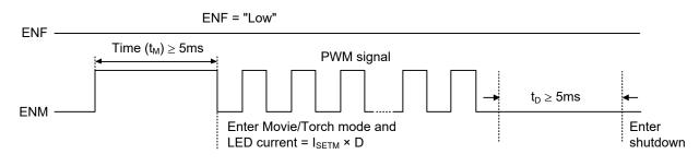
Figure 6. Timing Diagram of Movie/Torch Mode
