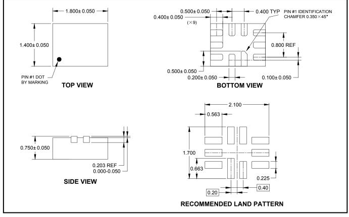
NOTE: All linear dimensions are in millimeters.
