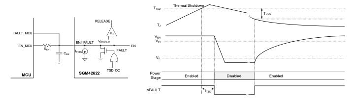
Figure 7. Thermal Shutdown in SGM42622
