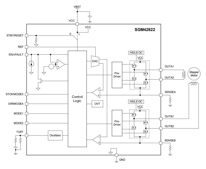
Figure 3. Block Diagram
