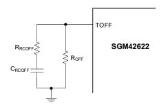
Figure 6. Programming PWM Off-Time
