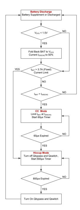
Figure 11. System Short Circuit Protection
