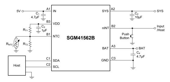
Figure 13. SGM41562B Typical Application Circuit with 5V Input
