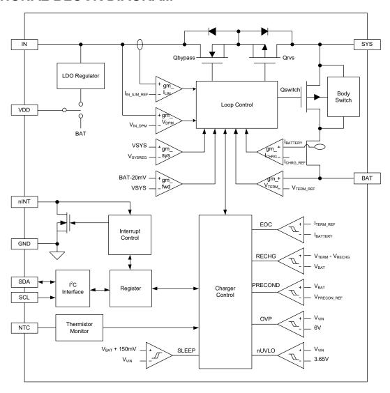
Figure 2. Functional Block Diagram
