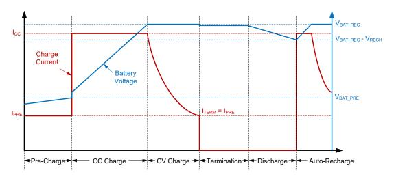
Figure 5. Battery Charge Profile
