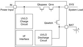
Figure 3. Power Path Management Structure
