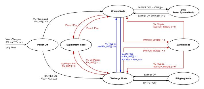
Figure 8. State Machine Conversion
