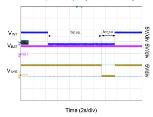
Figure 7. Power Recycling Waveforms
