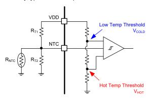
Figure 12. NTC Function Block
