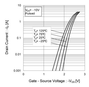
Fig.9 Gate Threshold Voltage vs.
