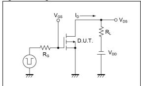
Fig.2-1 Gate Charge Measurement Circuit
