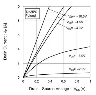
Fig.6 Typical Output Characteristics(II)
