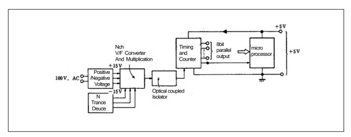
Figure 10. Connect to Micro Processor
