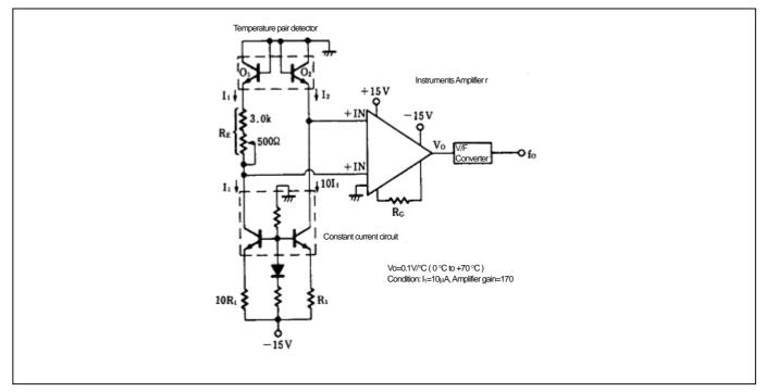
Figure 13. Temperature to Frequency converter
