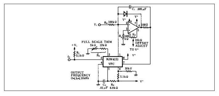
Figure 4. Precision Voltage-to-Frequency Converter
