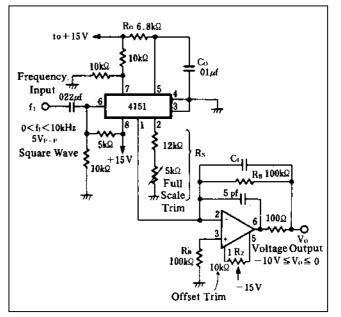
Figure 5. Single Supply Frequency-to-Voltage Converter
