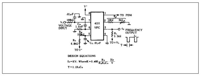
Figure 2. Single Supply Voltage-to-Frequency Converter
