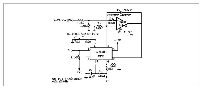
Figure 3. Precision Voltage-to-Frequency Converter Single Supply
