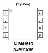
$\begin{array}{l} \mbox{PIN FUNCTION} \\ 1.I_o \ (Current Source) \\ 2.R_s \ (Scale Factor) \\ 3.V_{Lo} \ (Logic Output) \\ 4.GND \\ 5.R_o \ (One-Shot R,C) \\ 6.T_h \ (Threshold) \\ 7.V_i \ (Input Voltage) \\ 8.V_+ \end{array}$
