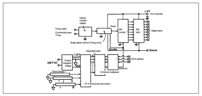
Figure 11. Multi channel ADC system
