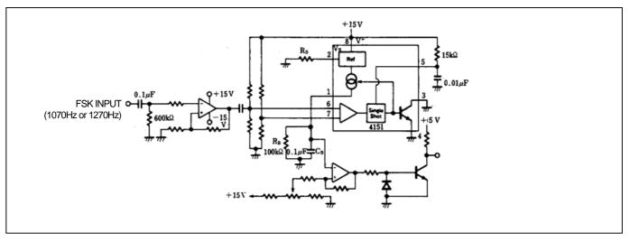
Figure 8. FSK demodulator
