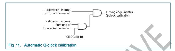
**Remark:** The duration of the automatic Q-clock calibration is 65 oscillator periods or approximately 4.8  $\mu$ s.
