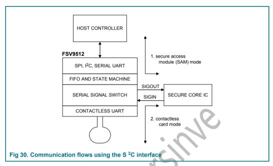
Configured in the Secure Access Mode the host controller can directly communicate to the Secure IC via SIGIN/SIGOUT. In this mode the FSV9512 generates the RF clock and performs the communication on the SIGOUT line. To enable the Secure Access module mode the clock has to be derived by the internal oscillator of the FSV9512, see bits SAMClockSel in register TestSel1Reg.
