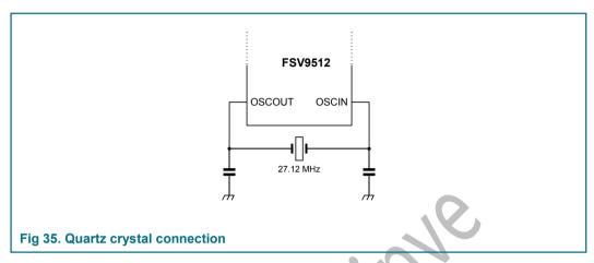
The clock applied to the FSV9512 provides a time basis for the synchronous system's encoder and decoder. The stability of the clock frequency, therefore, is an important factor for correct operation. To obtain optimum performance, clock jitter must be reduced as much as possible. This is best achieved using the internal oscillator buffer with the recommended circuitry.
