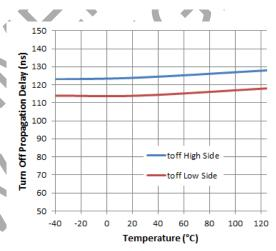
Figure 7. Turn-off Propagation Delay vs. Temperature
