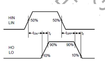
Figure 3. Switching Time Waveform Definitions
