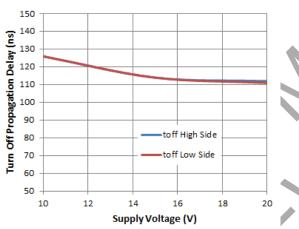
Figure 6. Turn-off Propagation Delay vs. Supply Voltage
