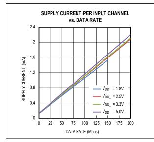
Figure 7. Supply Current Per Input Channel
