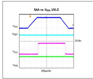
Figure 4. VDDA - UVLO Controlling SAA Signal
