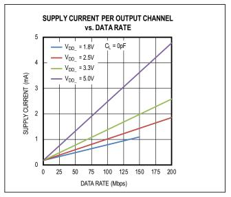
Figure 8. Supply Current Per Output Channel
