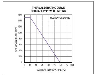
Figure 2. Thermal Derating Curve for Safety Power Limiting
