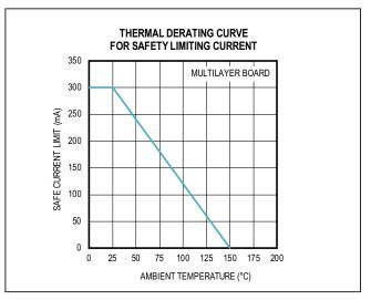
Figure 3. Thermal Derating Curve for Safety Current Limiting
