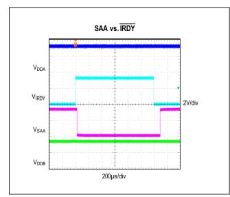
Figure 5. IRDY Controlling SAA Signal
