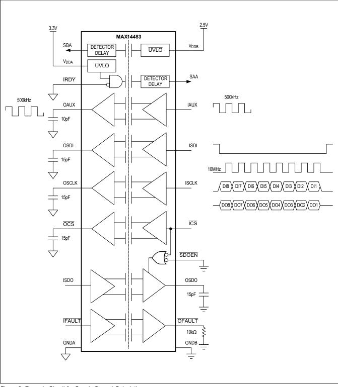
Figure 9. Example Circuit for Supply Current Calculation
