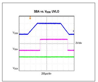
Figure 6. VDDB - UVLO Controlling SBA Signal
