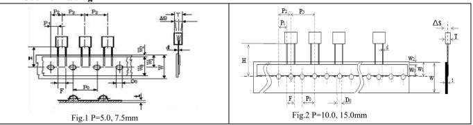
**▲** Taping Dimensions(mm)
