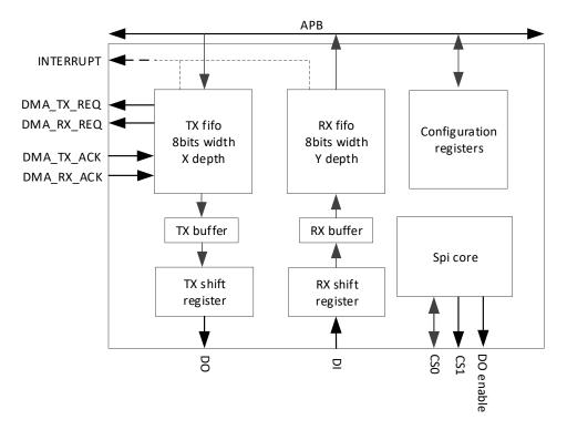
Figure 49: SPI Block Diagram
