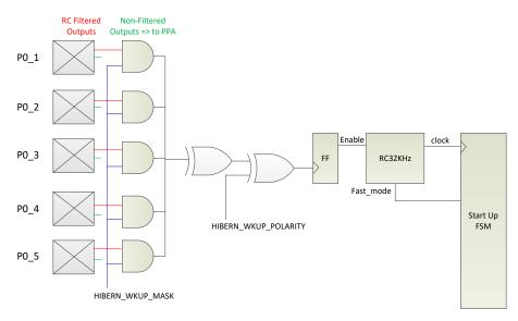
Figure 55: Clockless Wake-Up Controller Circuit
