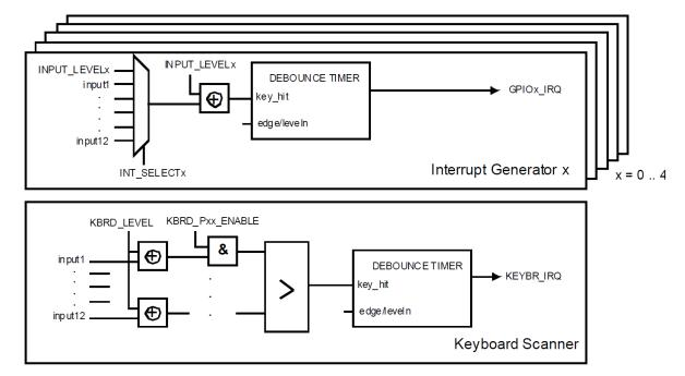
Figure 65: Keyboard Controller Block Diagram
