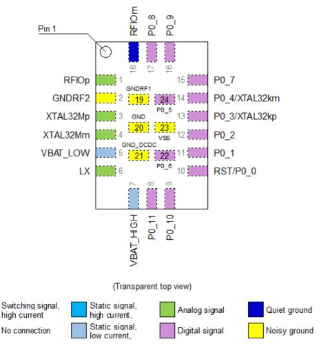
Figure 4: FCGQFN24 Pin Assignment (Top View)
