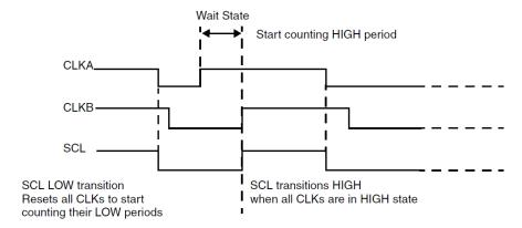
Figure 43: Multiple Master Clock Synchronization
