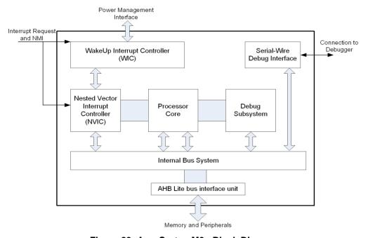
Figure 23: Arm Cortex-M0+ Block Diagram
