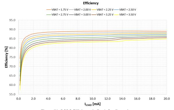
Figure 76: DCDC Efficiency in Buck Configuration
