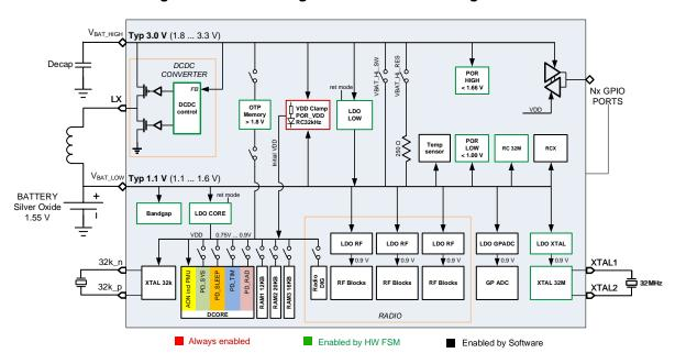
Figure 8: Power Management Unit: Boost Configuration
