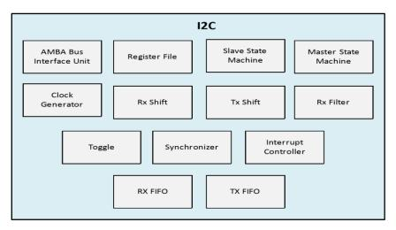
Figure 33: I2C Controller Block Diagram
