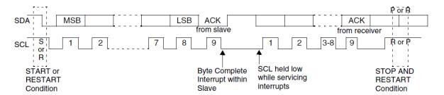
Figure 35: Data Transfer on the I2C Bus
