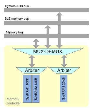
Figure 25: Memory Controller Block Diagram
