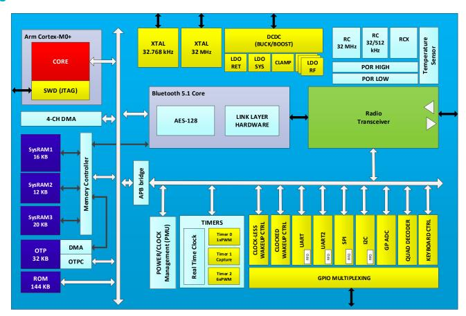
Figure 2: DA14531 Block Diagram
