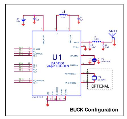
Figure 6: Buck Configuration System Diagram
