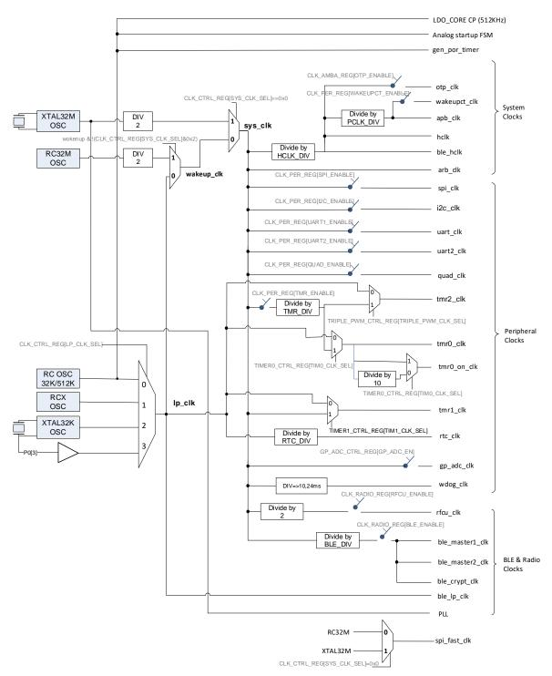
Figure 26: Clock Tree Diagram
