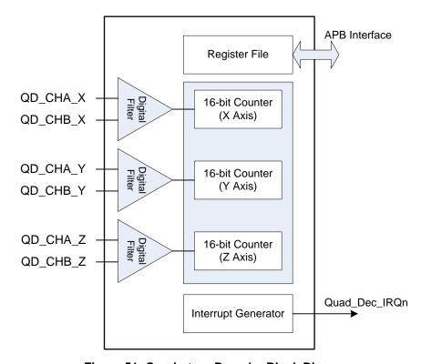
Figure 51: Quadrature Decoder Block Diagram
