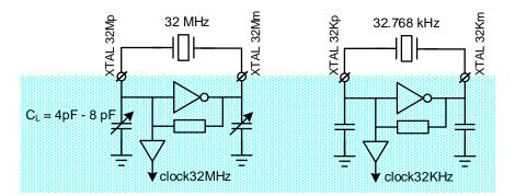
**Figure 27: Crystal Oscillator Circuits**
