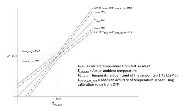
Figure 64: Temperature Sensor Behavior
