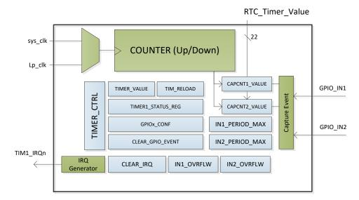
Figure 60: Timer 1 Block Diagram
