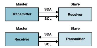
Figure 34: Master/Slave and Transmitter/Receiver Relationships
