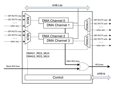
Figure 31: DMA Controller Block Diagram
