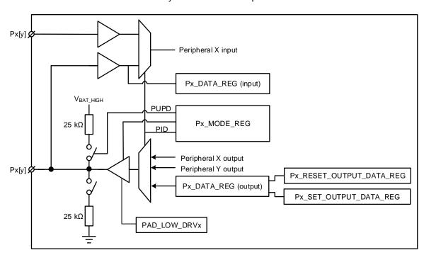
Figure 68: Port P0 with Programmable Pin Assignment and Driving Strength
