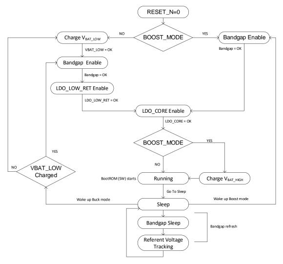
Figure 11: Power-Up/Wake-Up/Sleep FSM Diagram
