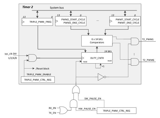
Figure 61: Timer 2 Block Diagram
