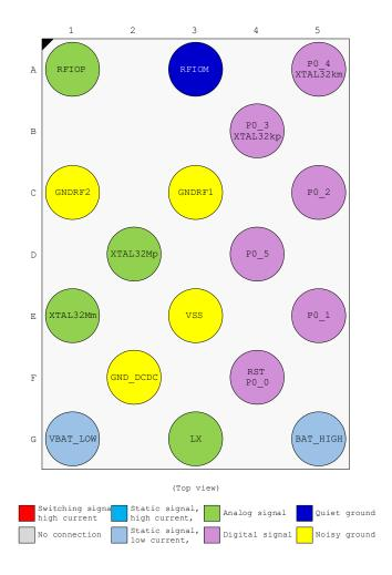
Figure 3: WLCSP17 Ball Assignment (Top View)
