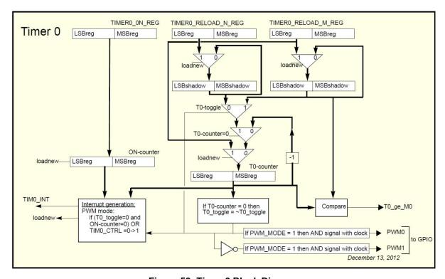
Figure 58: Timer 0 Block Diagram
