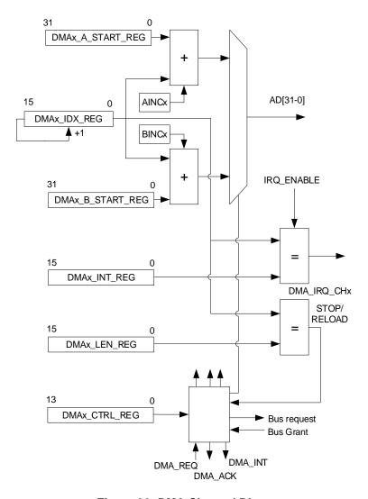
Figure 32: DMA Channel Diagram
