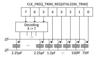
Figure 28: XTAL32MHz Oscillator Frequency Trimming
