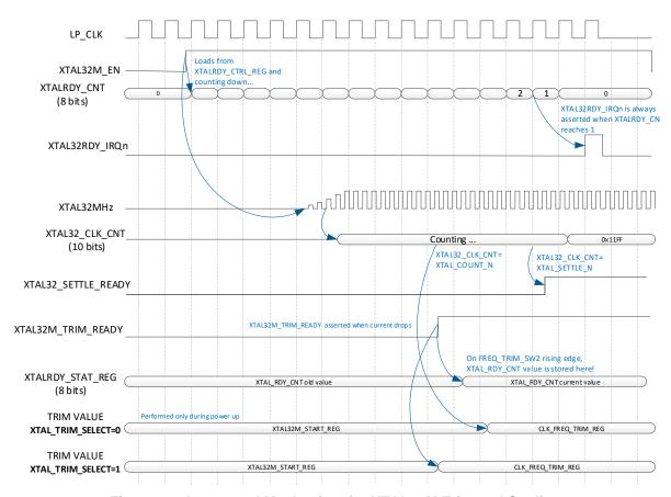
Figure 29: Automated Mechanism for XTAL32M Trim and Settling
