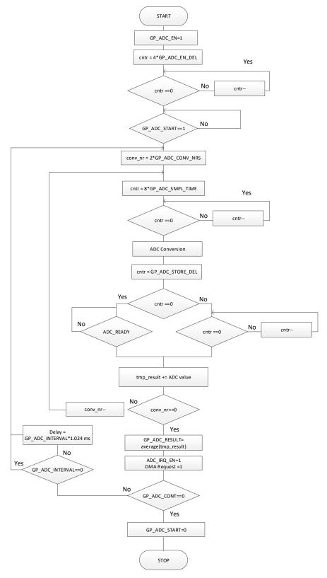
Figure 72: GPADC Operation Flow Diagram
