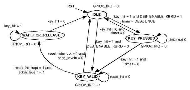
Figure 67: GPIO Interrupt Generator State Machine
