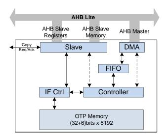
Figure 30: OTP Controller Block Diagram
