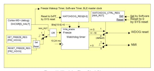
Figure 63: Watchdog Timer Block Diagram
