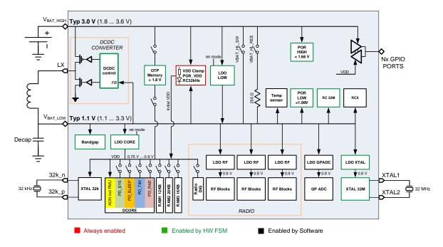
Figure 7: Power Management Unit: Buck Configuration
