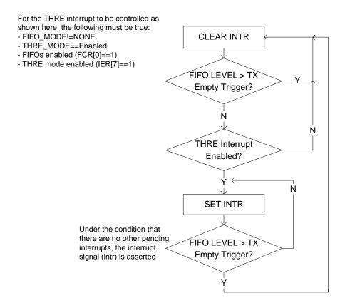
Figure 47: Flowchart of Interrupt Generation for Programmable THRE Interrupt Mode
