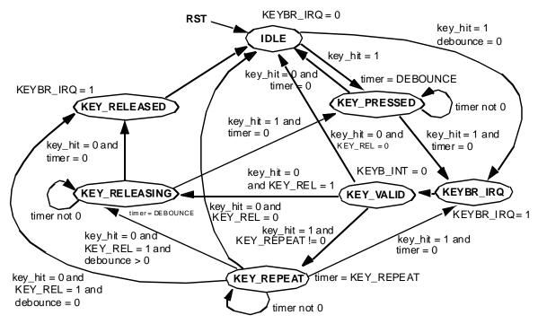
Figure 66: Keyboard Scanner State Machine
