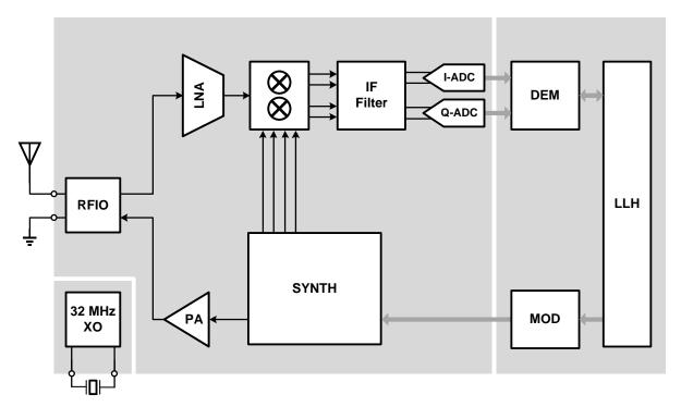
Figure 84: Bluetooth® Radio Block Diagram
