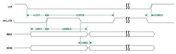
Figure 50: SPI Slave Mode Timing (CPOL = 0, CPHA = 0)
