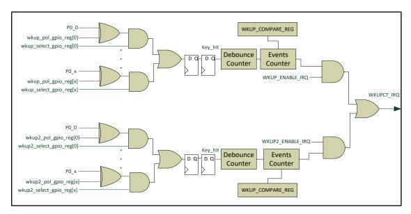
Figure 56: Clocked Wake-Up Controller Block Diagram
