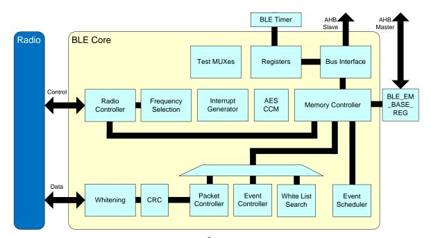
Figure 78: Bluetooth® LE Core Block Diagram
