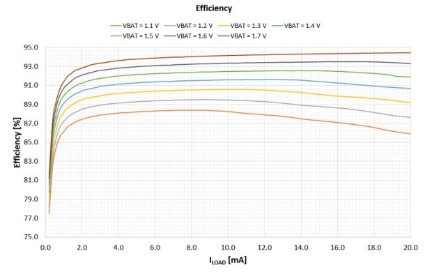
Figure 77: DCDC Efficiency in Boost Configuration
