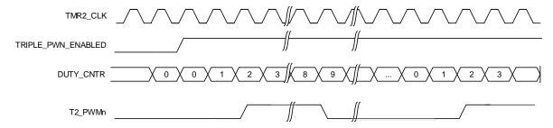
Figure 62: Timer 2 Timing Diagram
