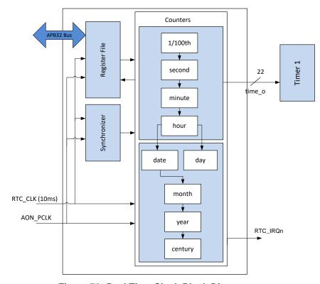
Figure 73: Real Time Clock Block Diagram
