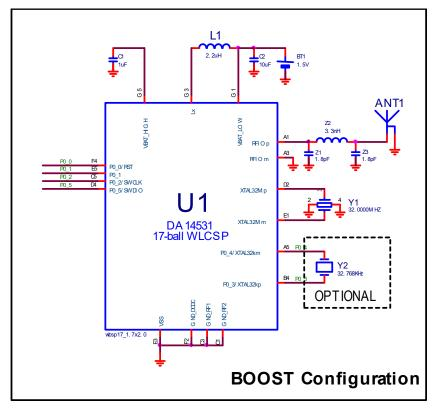
Figure 5: Boost Configuration System Diagram
