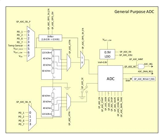
Figure 71: Block Diagram of GPADC
