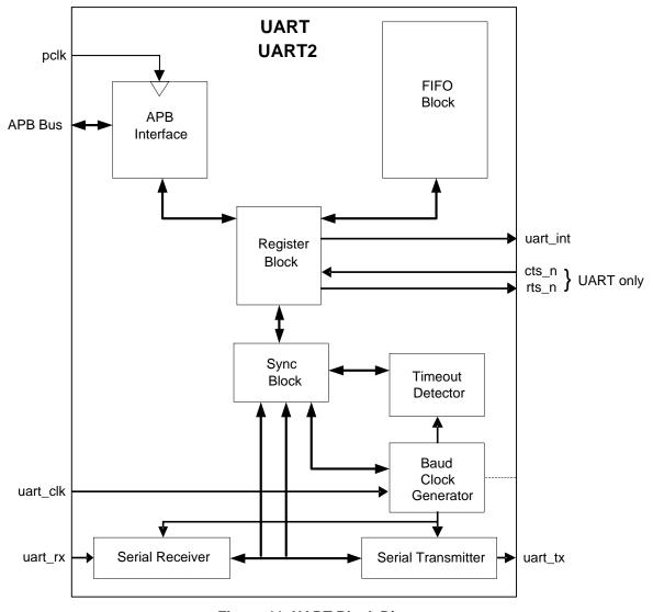
Figure 44: UART Block Diagram
