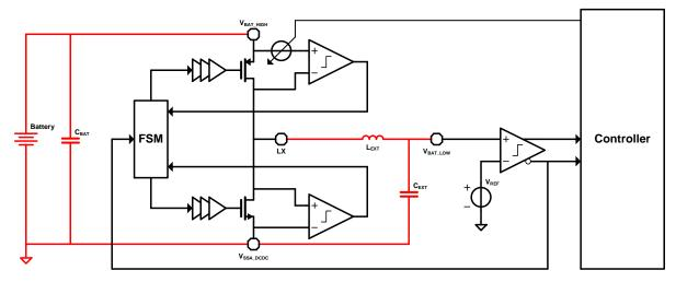
Figure 74: DCDC Block Diagram - Buck Configuration
