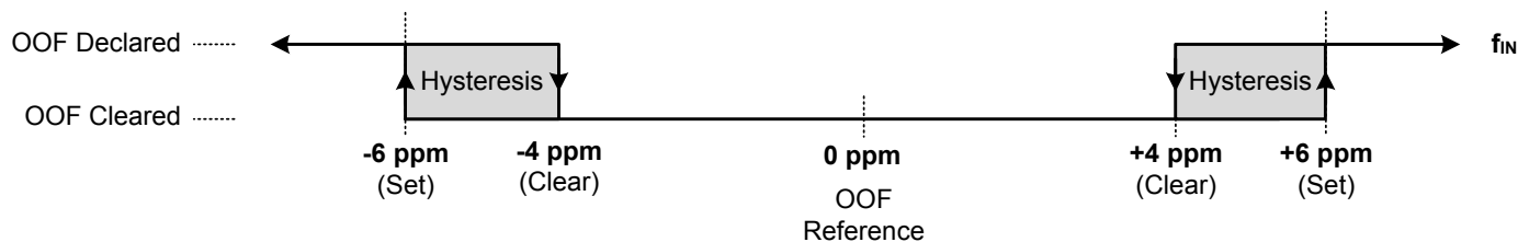
Figure 4.10. Example of Precise OOF Monitor Assertion and De-assertion Triggers
