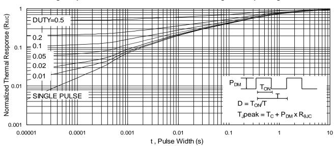
Fig.9 Normalized Maximum Transient Thermal Impedance
