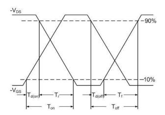
Fig.10 Switching Time Waveform
