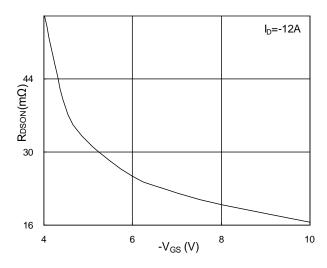
Fig.2 On-Resistance v.s Gate-Source
