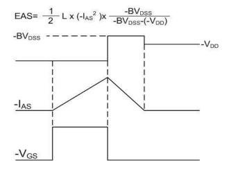
Fig.11 Unclamped Inductive Switching Waveform
