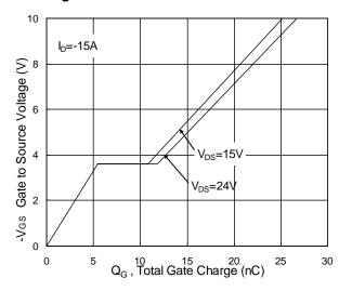
Fig.4 Gate-Charge Characteristics
