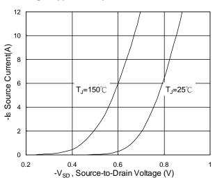
Fig.3 Forward Characteristics of Reverse
