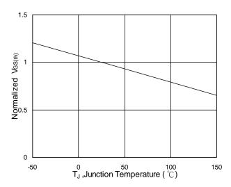
Fig.5 Normalized V<sub>GS(th)</sub> v.s T<sub>J</sub>
