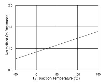
Fig.6 Normalized R<sub>DSON</sub> v.s T<sub>J</sub>
