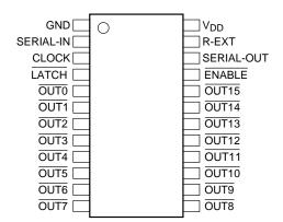
Warnings: Short-circuiting an output terminal toGND or to the power supply terminal may broken the device. Please take care when wiring the output terminals, the power supply terminal and the GND terminals.
