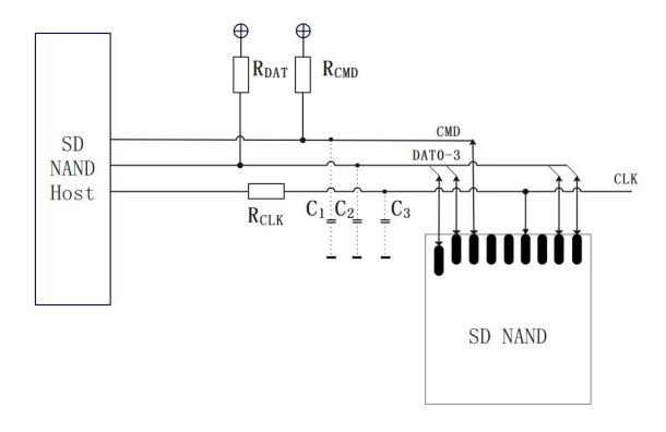
RDAT and RCMD (10K $\sim$ 100 k $\Omega$ ) are pull-up resistors protecting the CMD and the DAT lines against bus floating when SD NAND is in a high-impedance mode.
