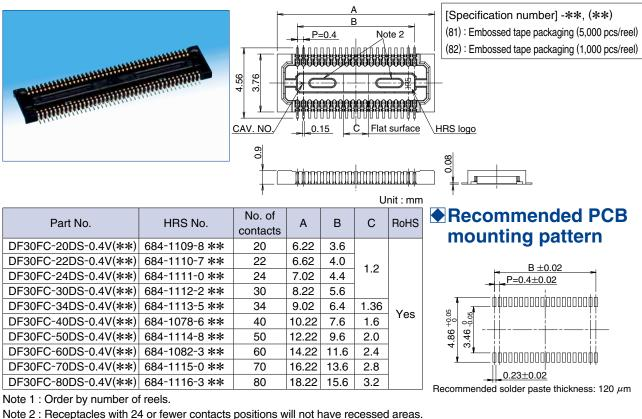
Header в [Specification number] -\*\*, (\*\*) P=0.4 (81) : Embossed tape packaging (5,000 pcs/reel) Note 2 Note 2 (82) : Embossed tape packaging (1,000 pcs/reel) 3.12 2.32 ċ HRS logo CAV. NO. Flat surface 0.15 0.8 0.08
