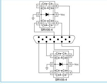
Figure 5 - Dual USB Port Protection
