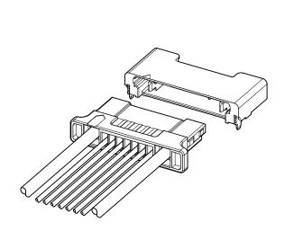
This connector is for connecting the lithium polymer battery or for connecting DC-IN, and has the sequence structure for connection to the power supply circuit in preference to connection to the signal circuit by dividing the signal circuit and power supply circuit clearly. Moreover, this is the low profile connector (space saving) for applying the high current by adopting the heat radiation structure.
