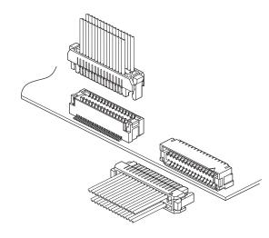
This is a wire-to-board connector for LVDS (Low Voltage Differential Signaling) interfaces inside digital display devices such as liquid crystal monitors and flat-screen TVs, which has excellent workability and robustness.
