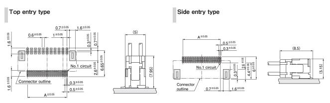
Note: 1. The figure of PC board layout is the figure viewed from the connector mounting side.
