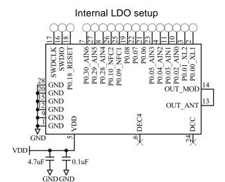
Internal LDO setup with external 32.768kHz X'tal
