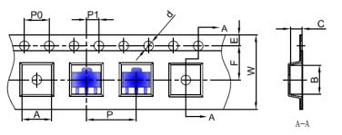
Packaging Description: SOT-89-3L parts are shipped in tape. The carrier tape is made from a dissipative (carbon filled) polycarbonate resin. The cover tape is a multilayer film (Heat Activated Adhesive in nature) primarily composed of polyester film, adhesive layer, sealant, and anti-static sprayed agent. These reeled parts in standard option are shipped with 1,000 units per 7" or 18.0 cm diameter reel. The reels are clear in color and is made of polystyrene plastic (anti-static coated).
