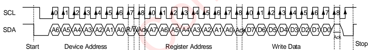
Figure 14 I 2 C Write Timing
