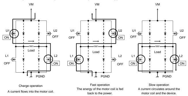
X In the timing of an output switching, the time to prevent a through current is predefined.
