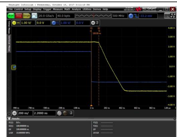
Voltage: 1V/div, Time: 200ns/div V_s = 5V , V_{IN} = 2V , R_L = \text{Open} , G = 3 Figure 24. Negative Overload Recovery
