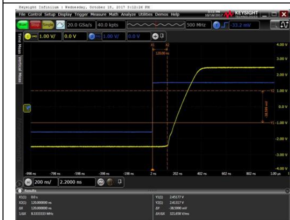
Voltage: 1V/div, Time: 200ns/div V_s = 5V , V_{IN} = 2V , R_L = \text{Open} , G = 3 Figure 23. Positive Overload Recovery
