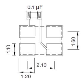
To ensure optimal oscillator performance, place a by-pass capacitor of 0.1uF as close to the part as possible between Vdd and GND pads.
