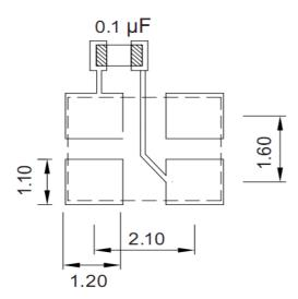
To ensure optimal oscillator performance, place a by-pass capacitor of 0.1uF as close to the part as possible between Vdd and GND pads.
