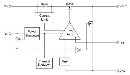
Figure 3. Block Diagram of FP6186
