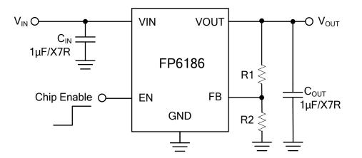
Figure 2. Typical Application Circuit for FP6186 adjustable voltage
