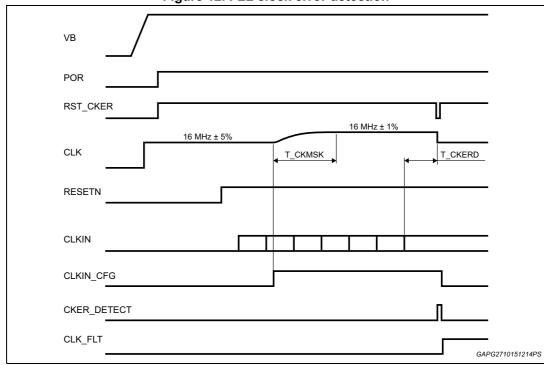
Figure 12. FLL clock error detection
