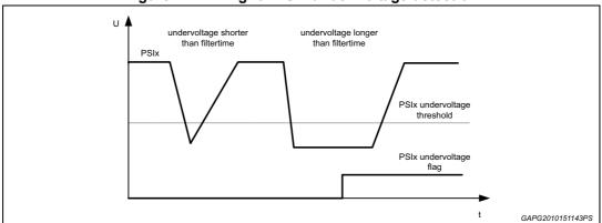
Figure 22. Timing for PSIx under voltage detection
