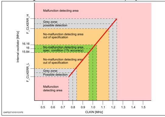
Figure 11. Internal oscillator vs external clock frequency
