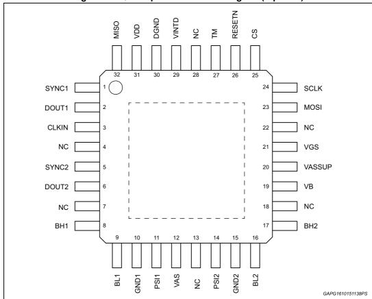
Figure 3. TQFP32 pins connection diagram (top view)
