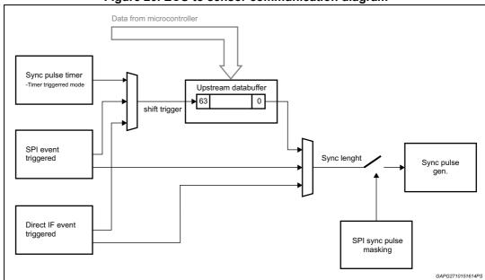
Figure 20. ECU to sensor communication diagram
