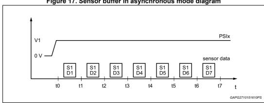
Figure 17. Sensor buffer in asynchronous mode diagram
