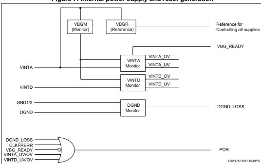
Figure 7. Internal power supply and reset generation
