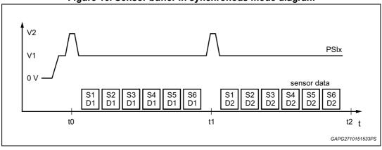
Figure 16. Sensor buffer in synchronous mode diagram
