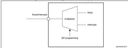
Figure 18. Block diagram with interrupt pins
