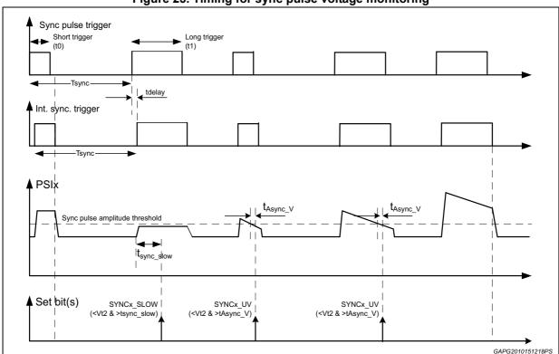
Figure 25. Timing for sync pulse voltage monitoring
