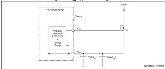
Figure 9. V<sub>AS</sub> application diagram
