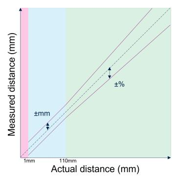
Figure 16. Ranging accuracy vs. distance
