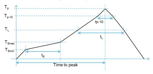
Note: The component should be limited to a maximum of three passes through this solder profile.
