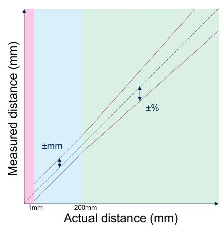
Figure 16. Ranging accuracy vs. distance
