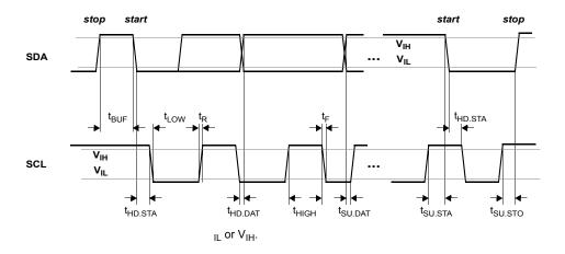
All timings are measured from either  $V_{\text{IL}}$  or  $V_{\text{IH}}.$
