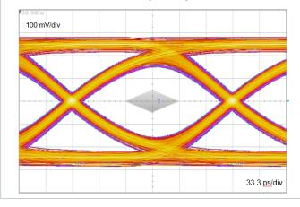
Figure 13. USB3.2 Gen1 – 5 Gbps Type-C eye diagram with device (with type C connector, reference cable and equalizer)
