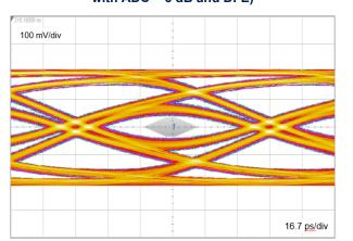
Figure 16. FPD LinkIII – 4.16 Gbps eye diagram without device
