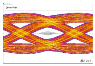
Figure 9. HDMI2.0 – 5.94 Gbps eye diagram with device (with worst cable and equaliser)
