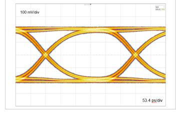
Figure 19. GMSL - 3.12 Gbps eye diagram with device
