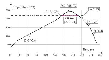
Minimize air convection currents in the reflow oven to avoid component movement. Maximum soldering profile corresponds to the latest IPC/JEDEC J-STD-020.
