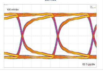
Figure 18. GMSL - 3.12 Gbps eye diagram without device
