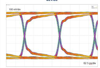
Figure 17. FPD LinkIII – 4.16 Gbps eye diagram with device
