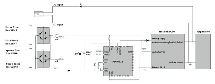
Figure 5-3. External Power Input Connected to PD70211 Output
