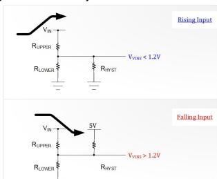
Figure 5-1. Equivalent Diagrams for UVLO and Hysteresis
