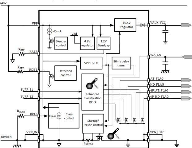
Figure 1-2. PD70211 Block Diagram (PWM Section)
