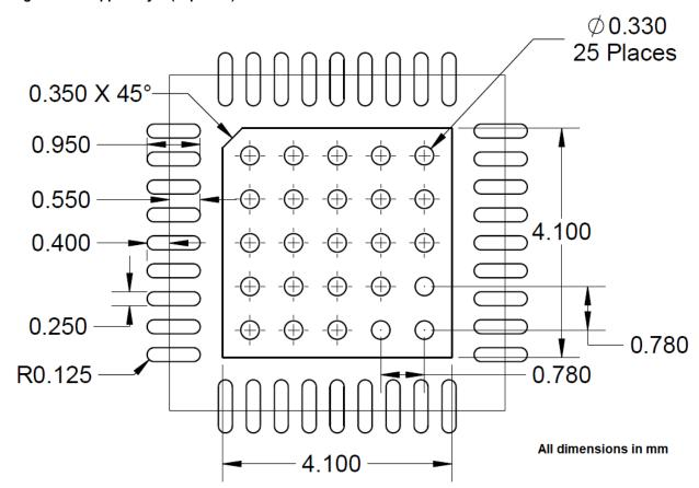
Figure 4-4. Paste Mask (Top View)
