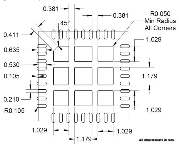
Note: Paste mask stencil is 5mil thick. All paste mask openings have a radius of 0.05 mm.
