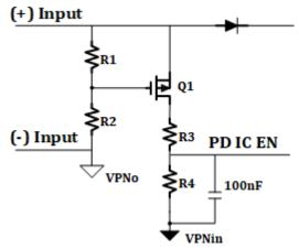
R1 and R2 set a rough threshold for PFET Q1 enable, to detect whether the external adapter exists or not. It must be set at a lower threshold than the PD70211 disable levels.
