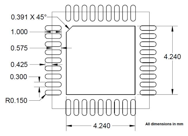
Figure 4-3. Copper Layer (Top View)
