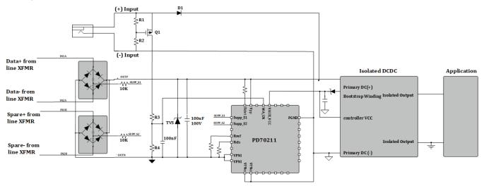
The PD70211 WA\_EN pin disables the Isolation switch and the PSE input power, when an external adapter is connected.
