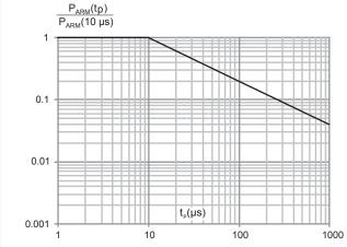
Figure 4. Relative variation of thermal impedance junction to ambient versus pulse duration (SMB)
