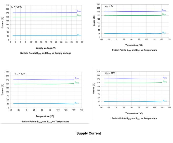
Output Switch Operate and Release Points (Magnetic Thresholds) – BOPS and BRPS
