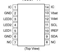
Figure 2. Pin Assignments
