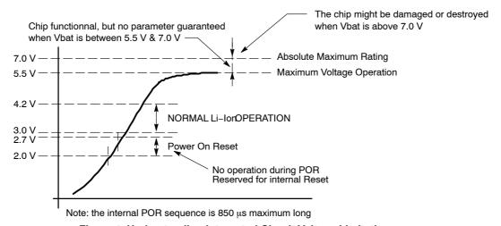
Figure 4. Understanding Integrated Circuit Voltage Limitations
