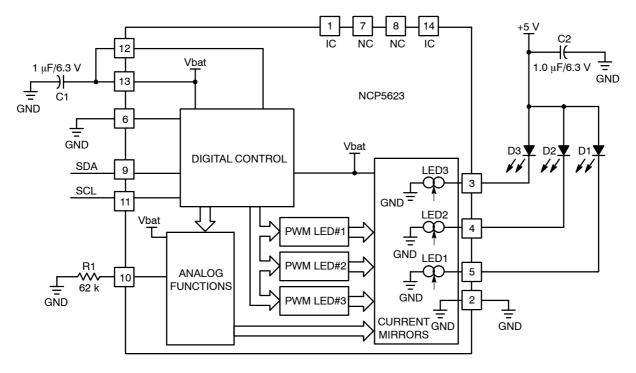
Figure 3. Simplified Block Diagram
