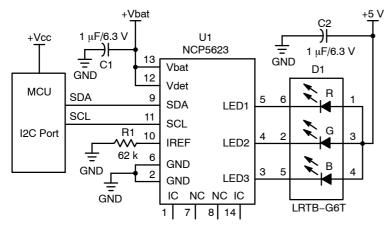
Figure 1. Typical Multiple Color LED Driver
