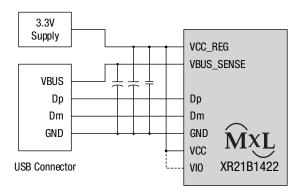
Figure 3: Self-Powered 3.3V Mode
