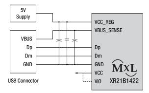
Figure 2: Self-Powered 5V Mode
