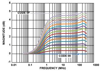
FIGURE 8. FREQUENCY RESPONSE vs 1MHz BITS 7:4
