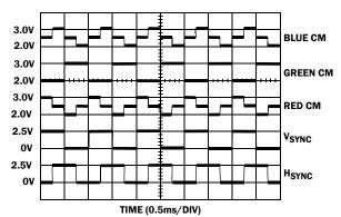
FIGURE 13. H AND V SYNC SIGNAL ENCODING
