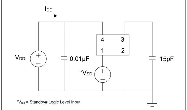
FIGURE 5-1: DSC1001/3/4 Test Circuit.
