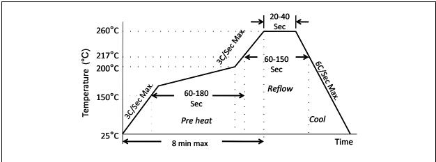
FIGURE 7-1: Solder Reflow Profile.
