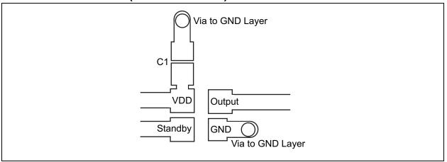
FIGURE 6-1: Recommended Board Layout for DSC1001/3/4.
