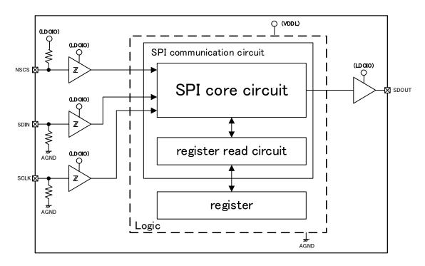
Fig. 5.7.a Block diagram for SPI communication circuit
