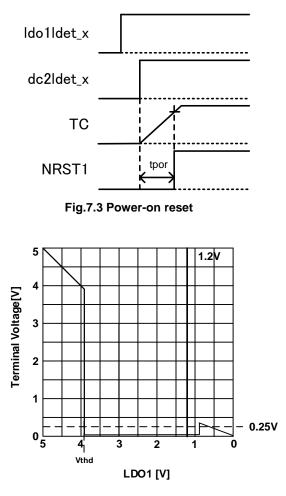
Fig.7.4 L retaining voltage
