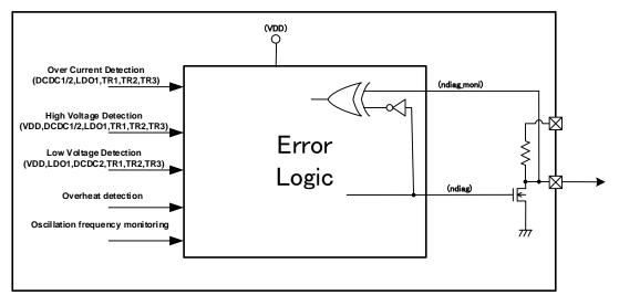
Error logic circuit block diagram
