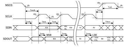
Fig.7.5 SPI Communication electrical characteristic
