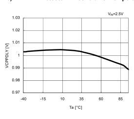
27) CPNDLY Detector Threshold vs. Temperature
