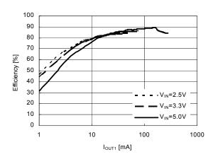
$f_{REQ}$  =1400kHz,  $V_{OUT}$ =12.0V
