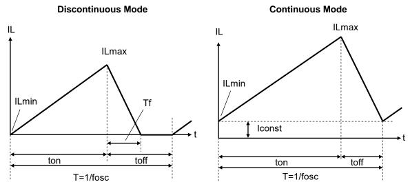
In PWM step-up DC/DC converter, there are two modes; the discontinuous mode and the continuous mode. These two modes depend upon the continuous characteristic of the inductor current.
