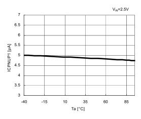
26) CPPDLY Detector Threshold vs. Temperature
