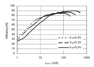
$f_{REQ}$  =210kHz,  $V_{OUT}$ =12.0V
