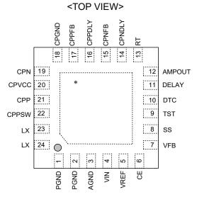
R1294L(QFN0404-24B) Pin Configuration
