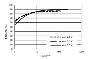
$f_{REQ}$  =700kHz,  $V_{OUT}$ =12.0V
