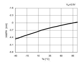
15) AMP"L"Output Current vs. Temperature
