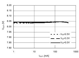
$f_{REQ} = 1400 \text{kHz}, V_{OUT} = 8.0 \text{V}$
