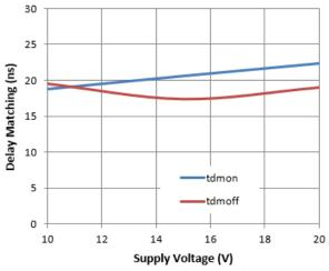
Figure 16. Delay Matching vs. Supply Voltage
