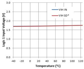
Figure 23. Logic 1 Input Voltage vs. Temperature
