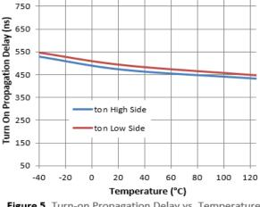
Figure 5. Turn-on Propagation Delay vs. Temperature
