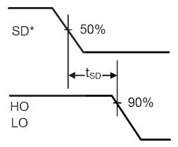
Figure 1. Input / Output Timing Diagram
