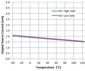
Figure 19. Output Source Current vs. Temperature
