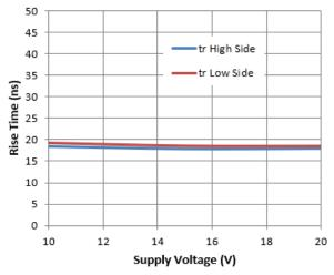
Figure 10. Rise Time vs. Supply Voltage
