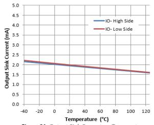
Figure 21. Output Sink Current vs. Temperature
