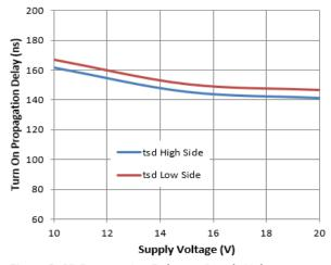
Figure 9. SD Propagation Delay vs. Supply Voltage
