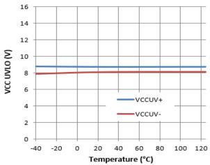
Figure 29. VCC UVLO vs. Temperature
