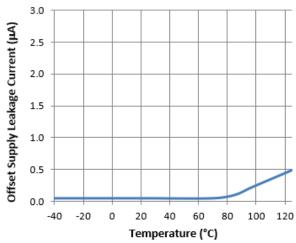
Figure 31. Offset Supply Leakage Current vs. Temperature
