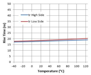
Figure 11. Rise Time vs. Temperature
