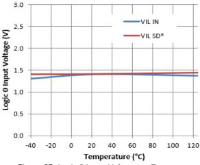
Figure 25. Logic 0 Input Voltage vs. Temperature
