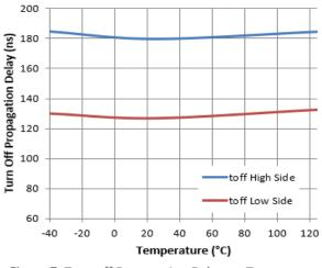
Figure 7. Turn-off Propagation Delay vs. Temperature
