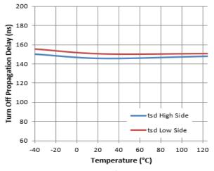
Figure 8. SD Propagation Delay vs. Temperature
