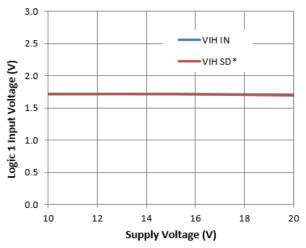
Figure 22. Logic 1 Input Voltage vs. Supply Voltage
