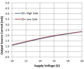
Figure 18. Output Source Current vs. Supply Voltage
