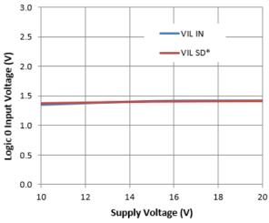
Figure 24. Logic 0 Input Voltage vs. Supply Voltage
