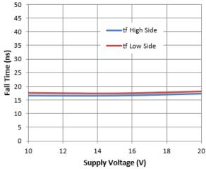
Figure 12. Fall Time vs. Supply Voltage
