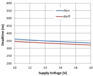
Figure 26. Deadtime vs. Supply Voltage
