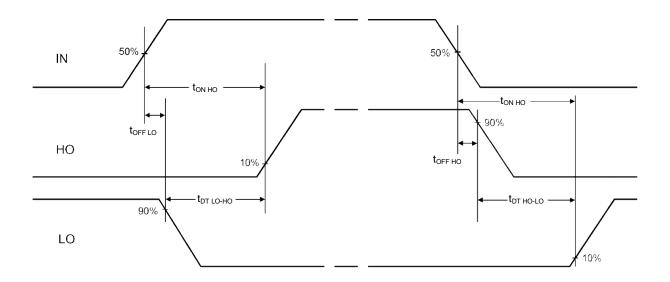
$\begin{array}{c} \text{Deadtime } t_{\text{DT LO-HO}} = t_{\text{ON HO}} \cdot t_{\text{OFF LO}} \\ t_{\text{DT HO-LO}} = t_{\text{ON LO}} \cdot t_{\text{OFF HO}} \\ \text{Deadtime matching} \\ t_{\text{MDT}} = t_{\text{DT LO-HO}} \cdot t_{\text{DT HO-LO}} \end{array}$
