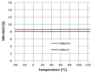
Figure 30. VBS UVLO vs. Temperature
