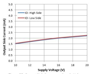
Figure 20. Output Sink Current vs. Supply Voltage
