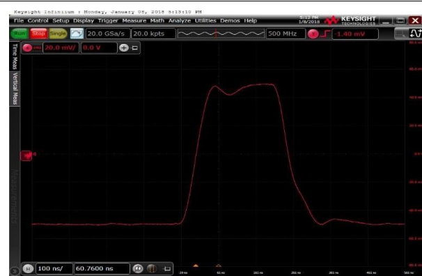
Voltage: 20mV/div, Time: 100ns/div V_s = \pm 15V , R_L = 2K , C_L = 100pF , G = 1 Figure 25. 100mV Signal Step Response
