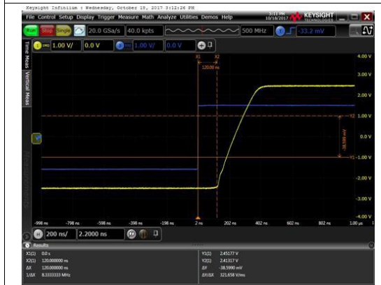
Voltage: 1V/div, Time: 200ns/div V_s = 5V, V_{IN} = 2V, R_L = \text{Open}, G = 3 Figure 23. Positive Overload Recovery
