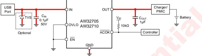
Figure 4 AW327XX typical application circuit(using default OVP threshold)
