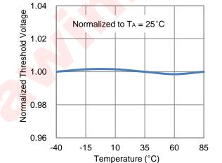
Figure 11 Normalized Internal OVP Threshold vs. Temp.
