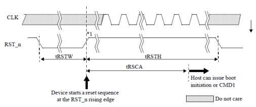
Figure 8. H/W reset waveform
