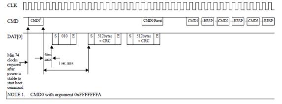
Figure 6. State diagram (alternative boot mode)
