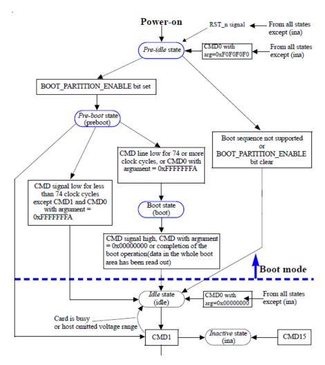
Figure 7. State diagram (boot mode) \*
