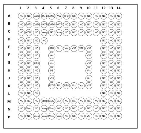
Figure 1. Ball Array (Top View through package)
