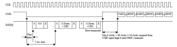
Figure 5. State diagram (boot mode)
