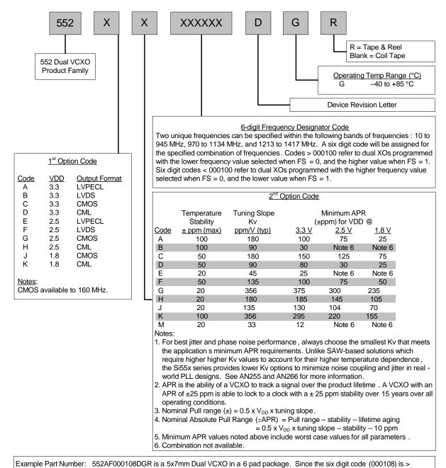
000100, f0 is 644.53125 MHz (lower frequency) and f1 is 693.48299 (higher frequency), with a 3.3V supply and LVPECL output. Temperature stability is specified as  $\pm$  50 ppm and the tuning slope is 135 ppm/V. The part is specified for a -40 to +85 C° ambient temperature range operation and is shipped in tape and reel format .
